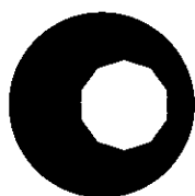
Field of view before Condenser alignment
