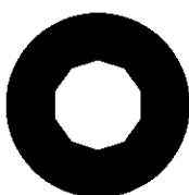
Field of view after Condenser alignment
